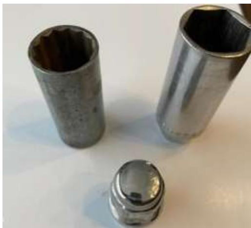
Regular sockets don’t work on cheap lug nuts
